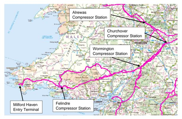
Figure 3 – Milford Haven and key compressor sites on the NTS.
