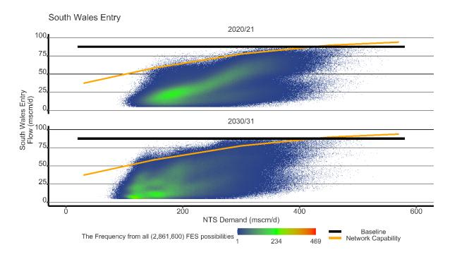
Figure 2 – Flame Chart illustration of existing NTS capability against entry capacity at Milford Haven ASEP
