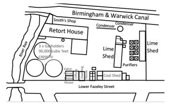
Figure 6. The layout of the Fazeley Street Gasworks based on an original drawing by Charles Hunt from 1902.
