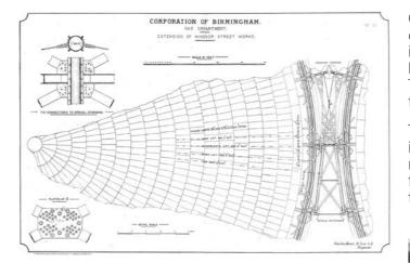
Figure 15. Extracts of the design of the giant twin gasholders built at Windsor Street, showing the interconnection between the two gasholders. Source: IGEM Archive.
