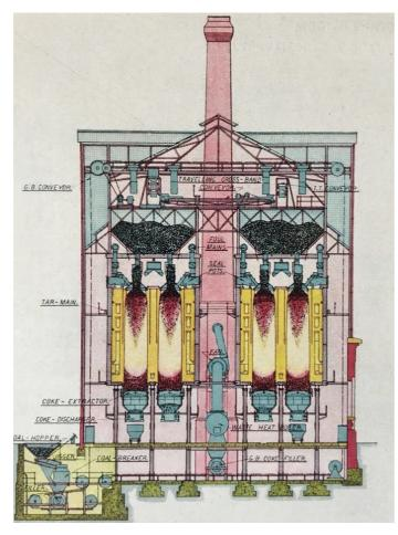
Figure 84. A drawing by Woodall Duckham of an installation of continuous vertical retorts. Source: IGEM Archive.
