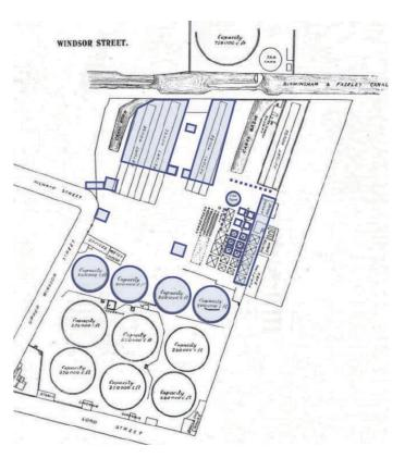
Figure 8. The plan of the Windsor Street Gasworks, in 1872, with the features which were present in 1854 shown in blue shading. Source: National Grid Gas Archive.
