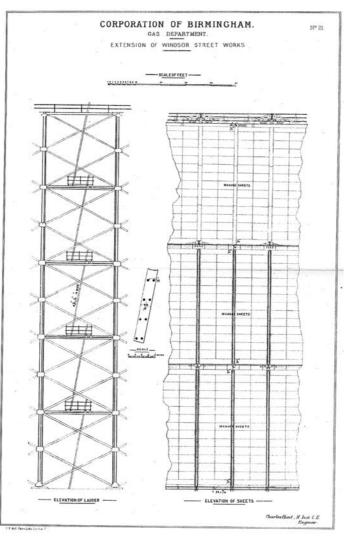
Figure 14. Extracts of the design of the giant twin gasholders built at Windsor Street, showing the frame and lifts. Source: IGEM Archive.
