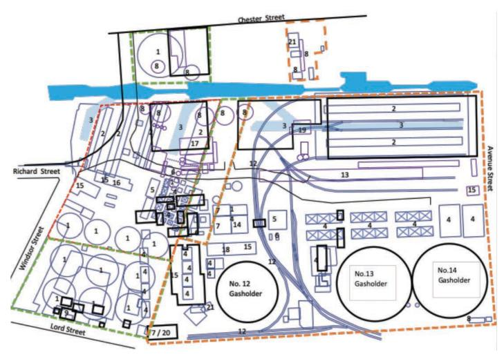
Figure 11. A plan of the whole Windsor Street Gasworks site, including the extensions undertaken by Charles Hunt, showing the main features. The early structures are in blue, later 20th Century additions are shown in purple. The plan is based on archive drawings obtained from the IGEM Archives and National Grid Archives. Key below:
