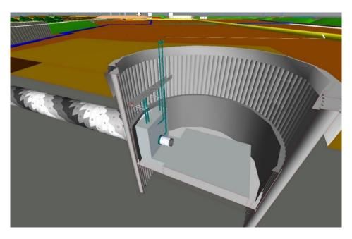
Figure 32: BIM image of TBM reception shaft
