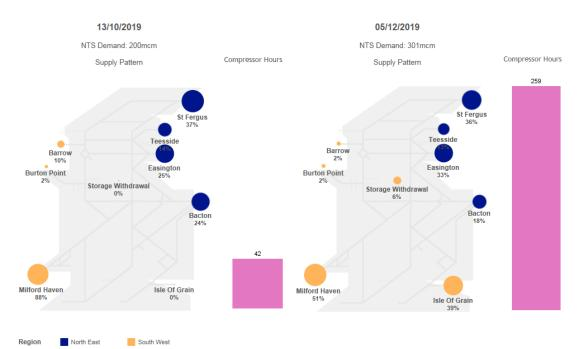
Figure 2: Compressor running hours and NTS demand on two separate days in the 2019/20 winter period.
