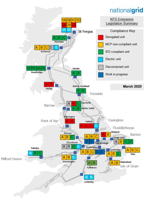
Figure 34: Compressor unit type and compliance with environmental legislation Peterborough and Huntingdon Compressor Stations (IPPC)
