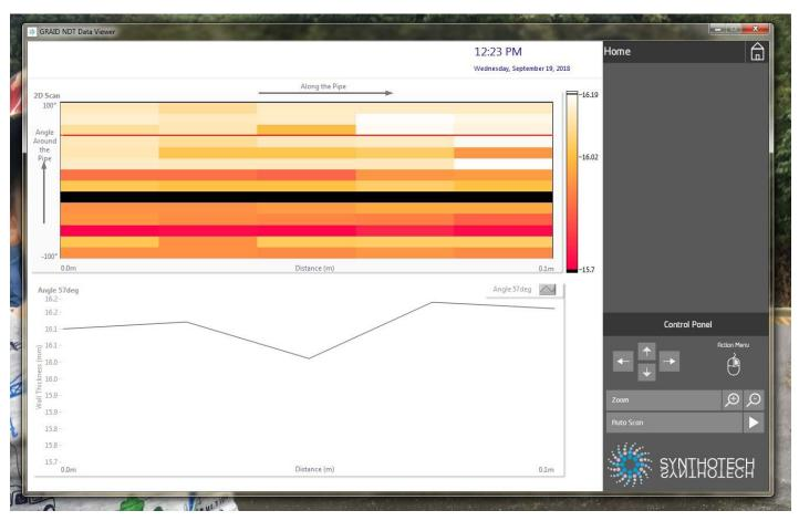
The EMAT testing sensors were used along the route, taking wall thickness readings in areas of interest.
