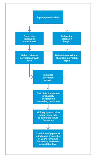
Figure 6 – Probabilistic corrosion growth model for calculating pipeline inspection interval.
