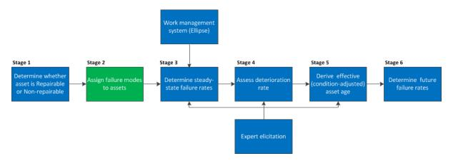
Figure 8 Overview of Sites defects/failure rate modelling approach
