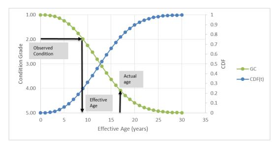
Figure 6 Using Condition / Asset Heath to calculate Effective Age
