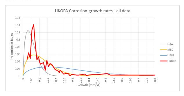
Figure 4 Modelled corrosion growth rates. Labels are corrosion rates, not corrosion resistance
