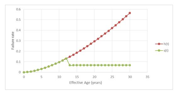
Figure 7 Failure rate models for secondary assets.
