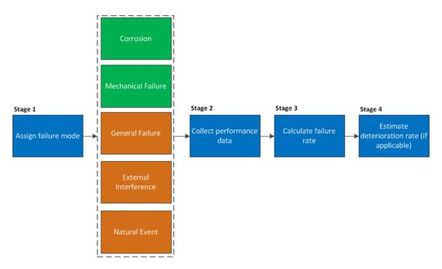
Figure 3 Overview of Pipelines defect/failure rate modelling approach
