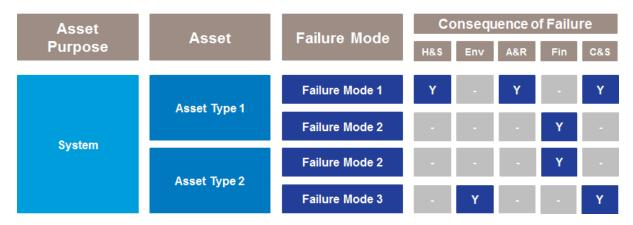
Figure 2 Mapping Asset Purpose to Failure Modes. Asset Types 1 & 2 has as shared FM (FM 2), but two different FM's (FM 1 and FM 3)
