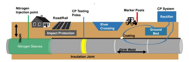
Figure 1 Relationships between Primary & Secondary assets in the Pipelines model
