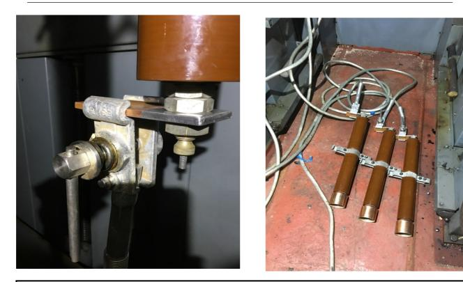
AS SHOWN (ABOVE LEFT) EARTH CLAMP CLAMPED TO SHORT COPPER BAR BOLTED TO THE BASE OF THE TEST BUSHING.
