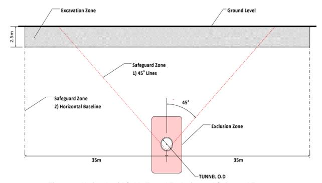
Figure 3 – National Grid Cable Tunnel Exclusion and Safeguard Zones
