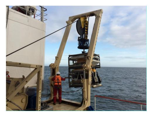
Figure 2: A Typical ROV being launched
