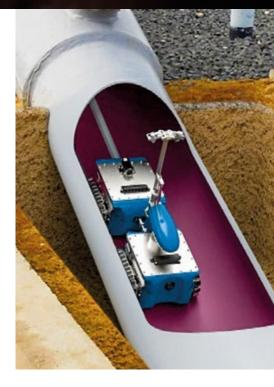
Pictures shown above GRAID robot developed for use in high-pressure underground gas pipelines.
