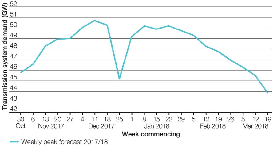
Figure 1.3 shows our current weekly transmission system demand peak forecasts for the coming winter. These are based on seasonal normal weather and are adjusted for normalised levels of embedded wind and solar generation.
