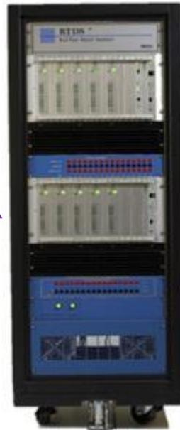
RTDS to perform flexible HiL tests
