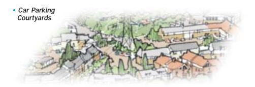
Car parking courtyards are used in the conceptual master plan around the base of pylons and work well in both residential and non-residential contexts. The need for access to pylons or for maintenance work on the overhead power lines needs to be taken into account.
