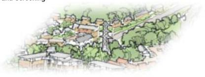
Appropriate planting can take place up to and underneath overhead power lines, reducing their visual impact and enhancing the overall environment. Attention needs to be paid to the precise species employed, the long-term management and the need to maintain appropriate safety clearances, as set out in appendix 3 and appendix 9. Within the conceptual master plan, strategic planting is used to screen distant views, as well as views from the immediate area around the pylons.
