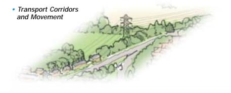
The conceptual master plan uses land beneath overhead power lines for streets and paths as part of a range of different uses to ensure the linearity of the route is not reinforced. Overhead power lines have less visual impact when seen from a moving vehicle than when seen from the same viewpoint by a pedestrian. Streets and paths also allow more landscaping to take place in the vicinity of the overhead power lines.
