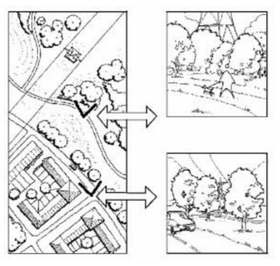
Planting at the base of pylons can reduce the impact at the pedestrian level.
