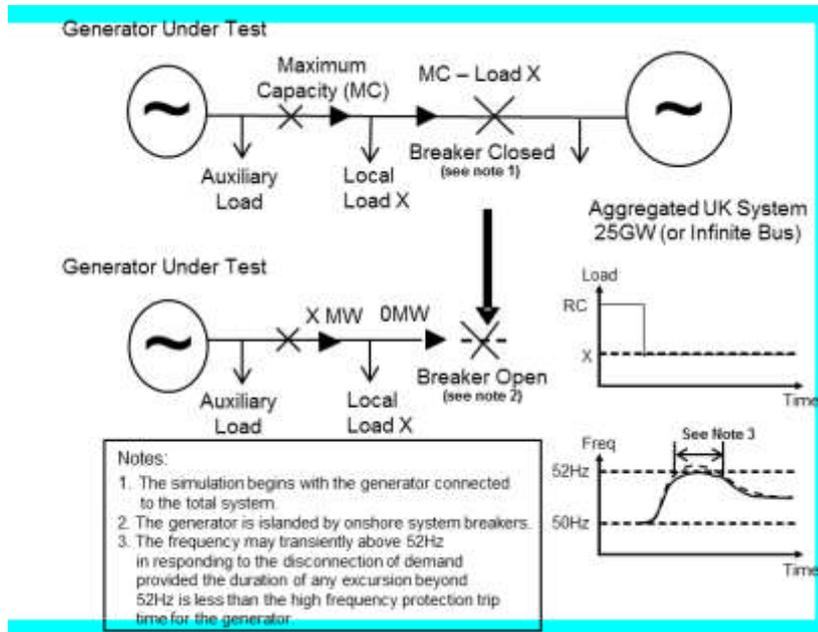
Figure ECP.A.3.6.1 – Diagram of Load Rejection Study
