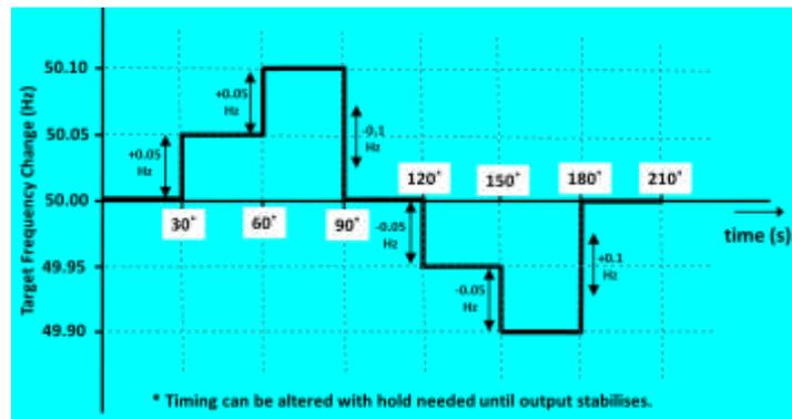
ECP.A.7.5. Figure 3 – Target Frequency setting changes
