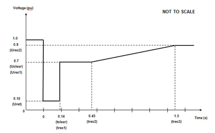
Figure ECC.6.3.15.3 - Voltage against time curve applicable to **Type C and D Synchronous Power Generating Modules** connected below 110kV
