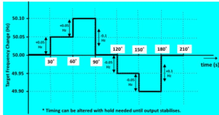
ECP.A.5.8 Figure 3 – Target Frequency setting changes
