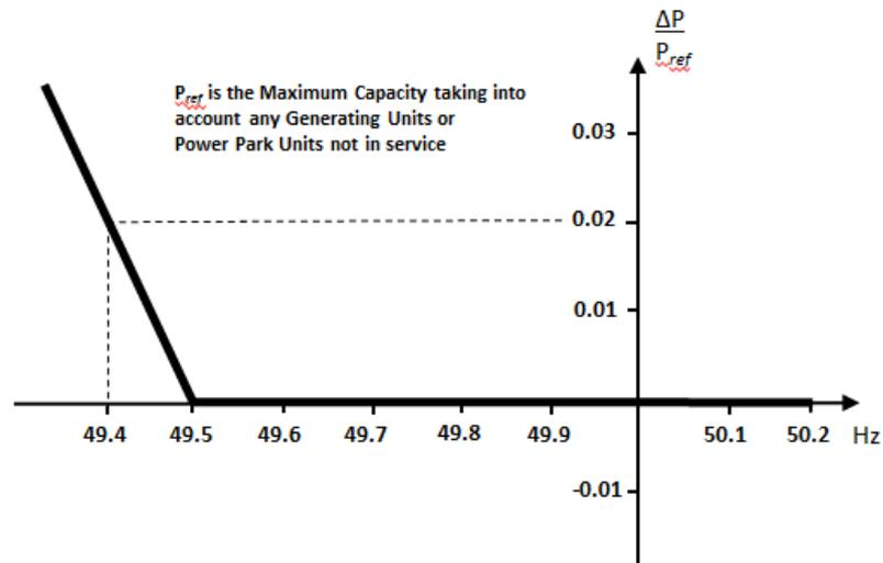
Figure ECC.6.3.7.2.2 –  $P_{ref}$  is the reference Active Power to which  $\Delta P$  is related and  $\Delta P$  is the change in Active Power output from the Power Generating Module (including DC Connected Power Park Modules) or HVDC System. The Power Generating Module (including DC Connected Power Park Modules or HVDC Systems) has to provide a positive Active Power output change with a droop of 10% or less based on Pref.
