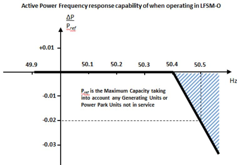
Figure ECC.6.3.7.1 –  $P_{ref}$  is the reference **Active Power** to which  $\Delta P$  is related and  $\Delta P$  is the change in **Active Power** output from the **Power Generating Module** (including **DC Connected Power Park Modules**) or **HVDC System**. The **Power Generating Module** (including **DC Connected Power Park Modules** or **HVDC Systems**) has to provide a negative **Active Power** output change with a droop of 10% or less based on  $P_{ref}$ .
