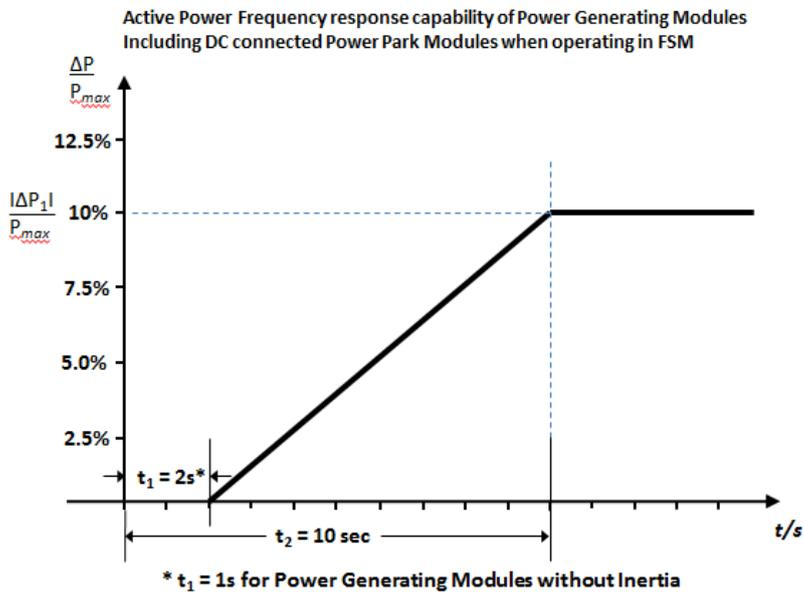
Figure 6.3.7.3.3(b) Active Power Frequency Response capability.
