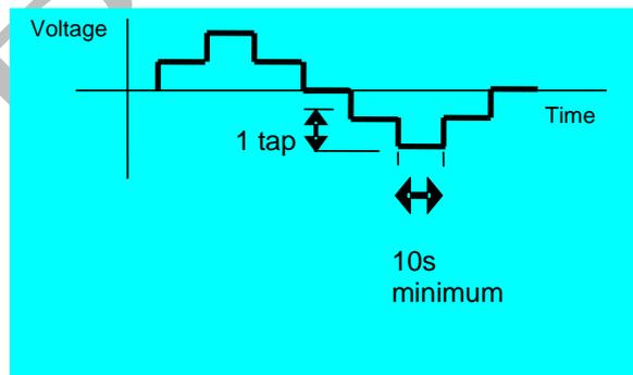
ECP.A.7.4 Figure 1 – Transformer tap sequence for voltage control tests
