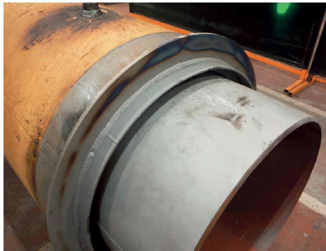
A nitrogen sleeve comprises a sealed steel shell that’s pressurised with nitrogen to protect it against corrosion on the inside of the shell.
