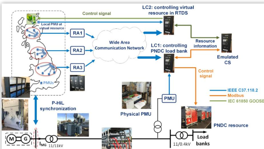
Figure 9. Schematic of the wide-area operation mode test configuration
