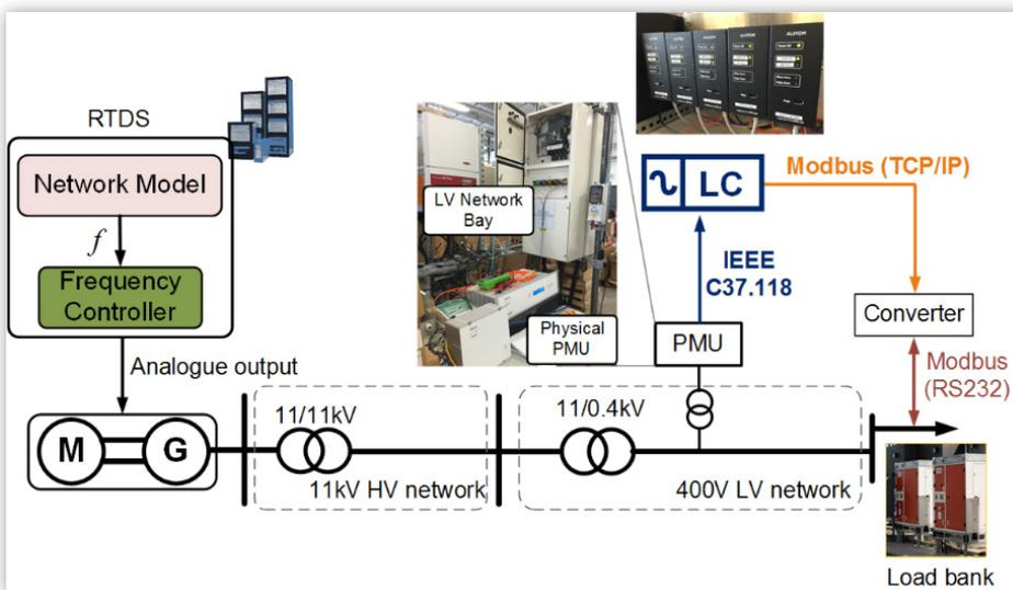
Figure 8. Schematic of the local operation mode test configuration
