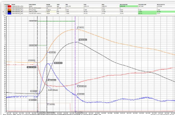
Figure 5. Plot of revised frequency control logic response (blue line) to an actual system event compared to existing frequency control logic response (black line)
