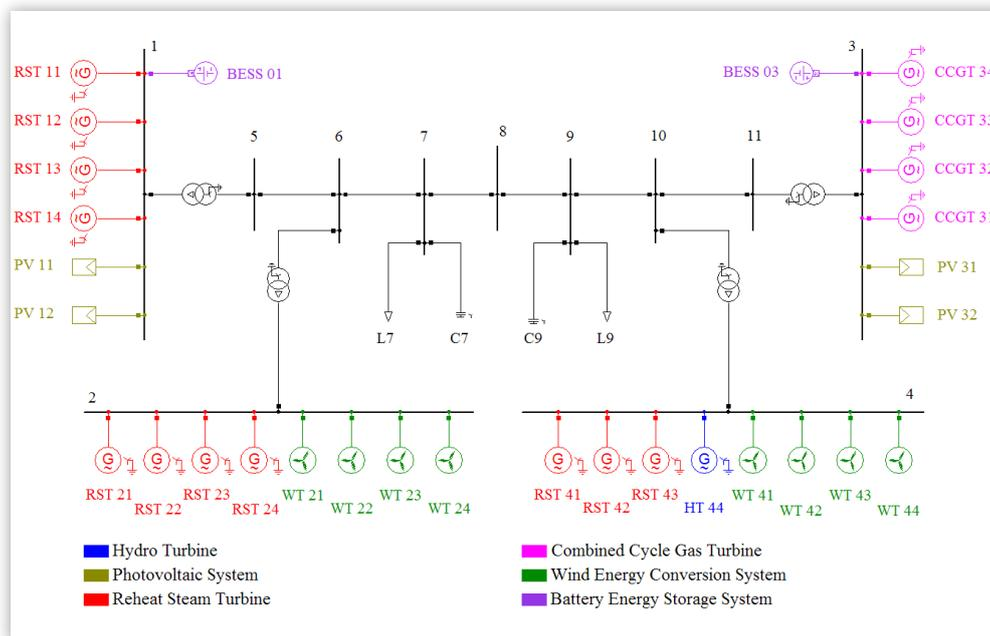
Figure 6. Single line diagram of the two-area system in DlgSILENT PowerFactory
