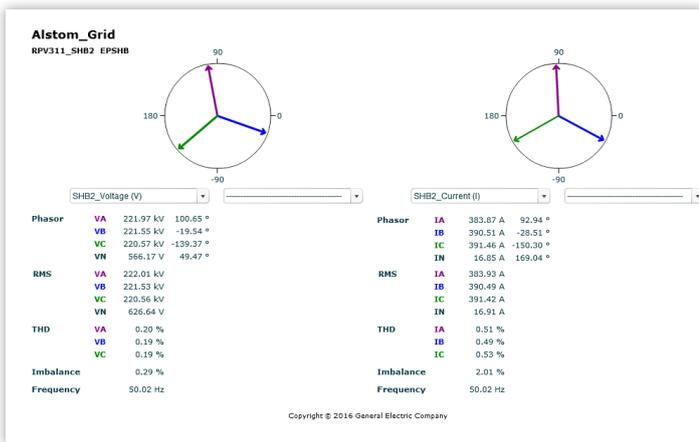
Figure 4. PMU readings of voltages and currents measured at South Humber Bank 400kV substation
