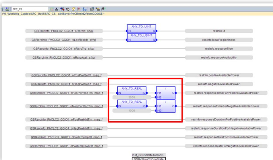
Figure 7. Additional logic added to the central supervisor
