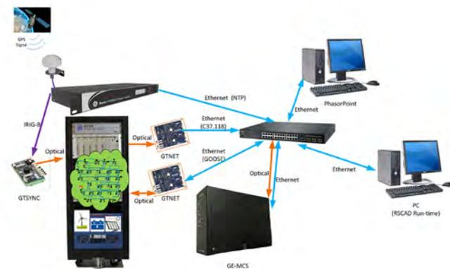
Figure 5: RTDS-HiL testbed and communication setup
