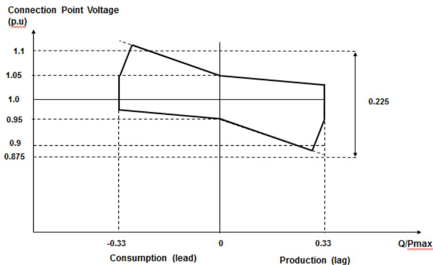
**Voltage/ Reactive Capability diagram for a Type C or D Power Park Module with a Connection Point at or below 33kV (NB most would be Distribution-connected):**
