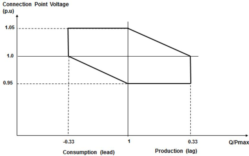
**U-Q/Pmax profile for a Type C or D Power Park Module with a Connection Point at or below 33kV (NB most would be Distribution-connected):**
