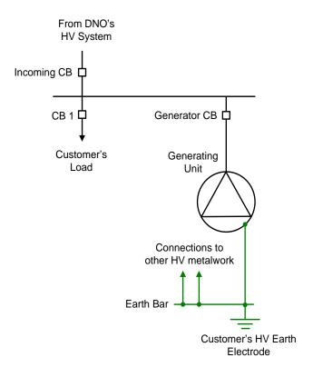
(1) Generating Unit winding is not connected to earth irrespective of whether it is star or delta connected
