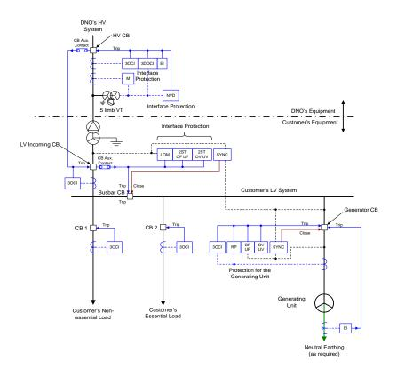
**Figure 10.5** - Typical Protection Diagram for an **LV Generating Unit** Connected to a **DNO LV System** Designed for Parallel Operation Only
