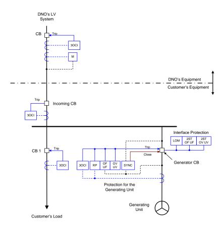
**Figure 10.6** - Figure 10.6 - Typical Protection Diagram for an **LV Generating Unit** Connected to a **DNO LV System** Designed for both Independent Operation (ie Standby Operation) and Parallel Operation
