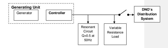
The directly coupled Generating Unit is to be tested at three levels of the
