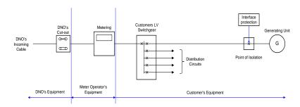
Fig 11.2 - Example of a Operational Diagram
