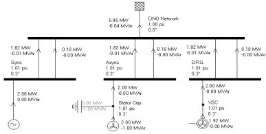
Figure 5 - Impedance Step Change Network
