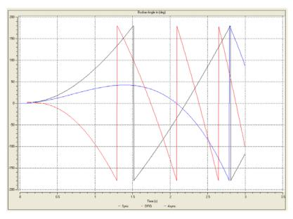
Figure 3 Voltage Angle (flips at +/- 180 Deg)
