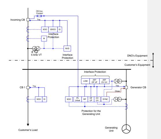
**Figure 10.3** - Typical Protection Arrangement for an **HV Generating Unit** Connected to a **DNO HV System** Designed for both Independent Operation (ie Standby Operation) and Parallel Operation
