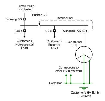
(1) Interlocking between busbar CB and  ${\bf Generator}$  CB is required to prevent parallel operation of the  ${\bf Generating}$   ${\bf Unit}$  and  ${\bf DNO}$   ${\bf System}$
