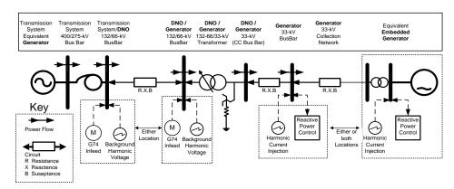
Fig 6.1 Example equivalent Total System representation
