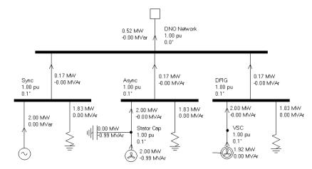
Figure 1 - Three Generator types
