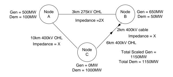
Assuming Node A is the reference node<sup>†</sup>, each 400kV circuit has impedance X, the 275kV circuit has impedance 2X, the 400kV cable circuit expansion factor is 10 and the 275kV overhead line circuit expansion factor is 2, the DCLF transport algorithm calculates the base case power flows for Peak Security background as follows:
