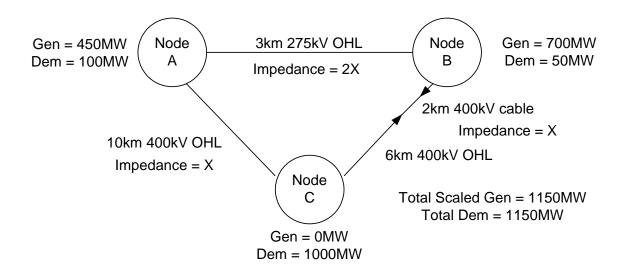
Assuming the same circuit impedances and expansion factors as used above in the Peak Security background, the DCLF transport algorithm calculates the base case power flows for Year Round background as follows:
