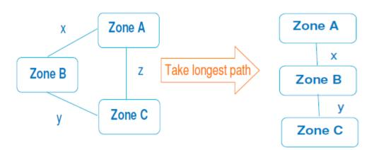
• Parallel zones – parallel zones will be amalgamated with the incremental km immediately beyond the amalgamated zones being the greater of those existing prior to the amalgamation. An illustrative example is shown below with a, b, c, and d representing the the initial incremental km between zones, and x and y representing the final incremental km following zonal amalgamation.
