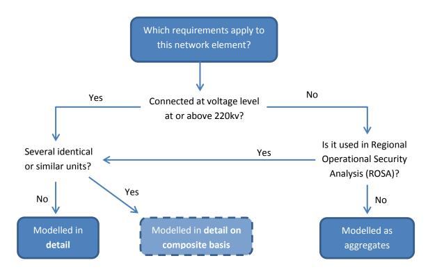
Generation may be modelled in detail, on a composite basis. For example a wind farm may be modelled as a single generator even if in reality it is composed of many similar individual units.
