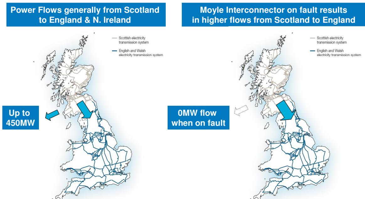
**Figure 1: Overview of power flows with and without the Moyle Interconnector**
