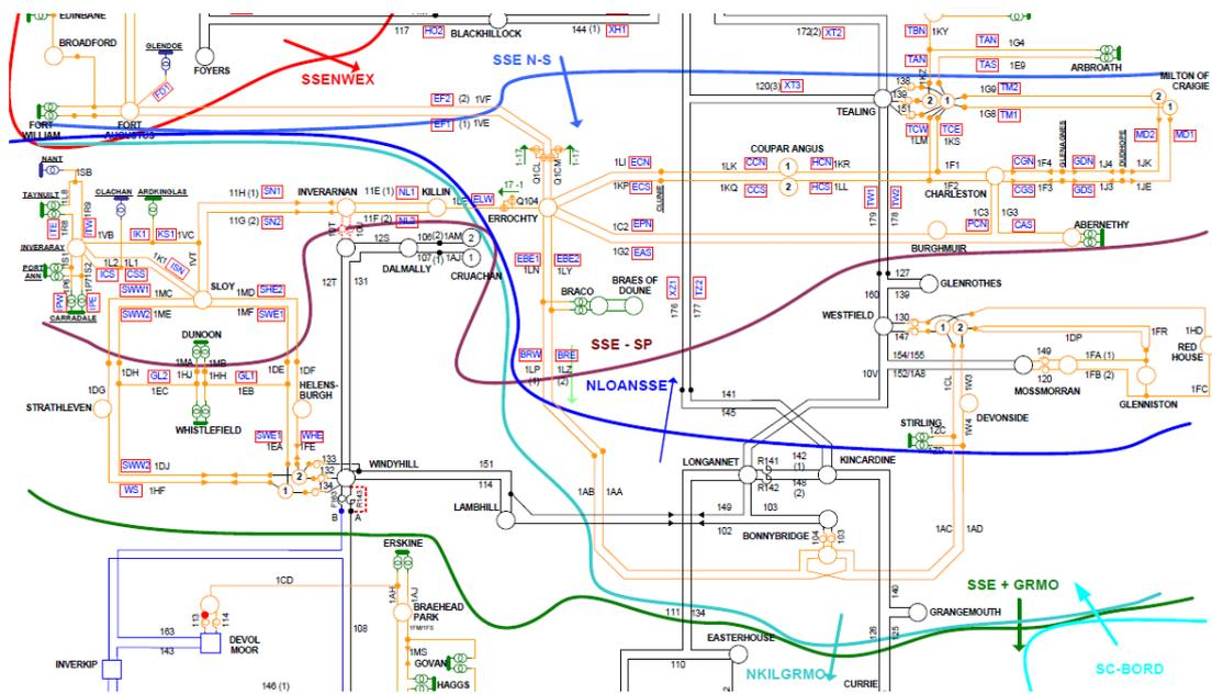
144. SSE –SP boundary is not typically used in Operational timescales as a boundary to describe a specific issue in more detail would be preferred. For modelling purposes, it can be used to adequately describe issues associated with the loss of a 275kV route against a combination of Peterhead and all northern wind generation.
