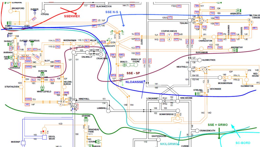
146. System instability constrains the transfer that can be secured across this boundary. The transfer that can be secured across this boundary is heavily dependant on the number of Longannet generators synchronised and the output of each generator. This is modelled by considering only the output of generation at Longannet and using the corresponding limit.
