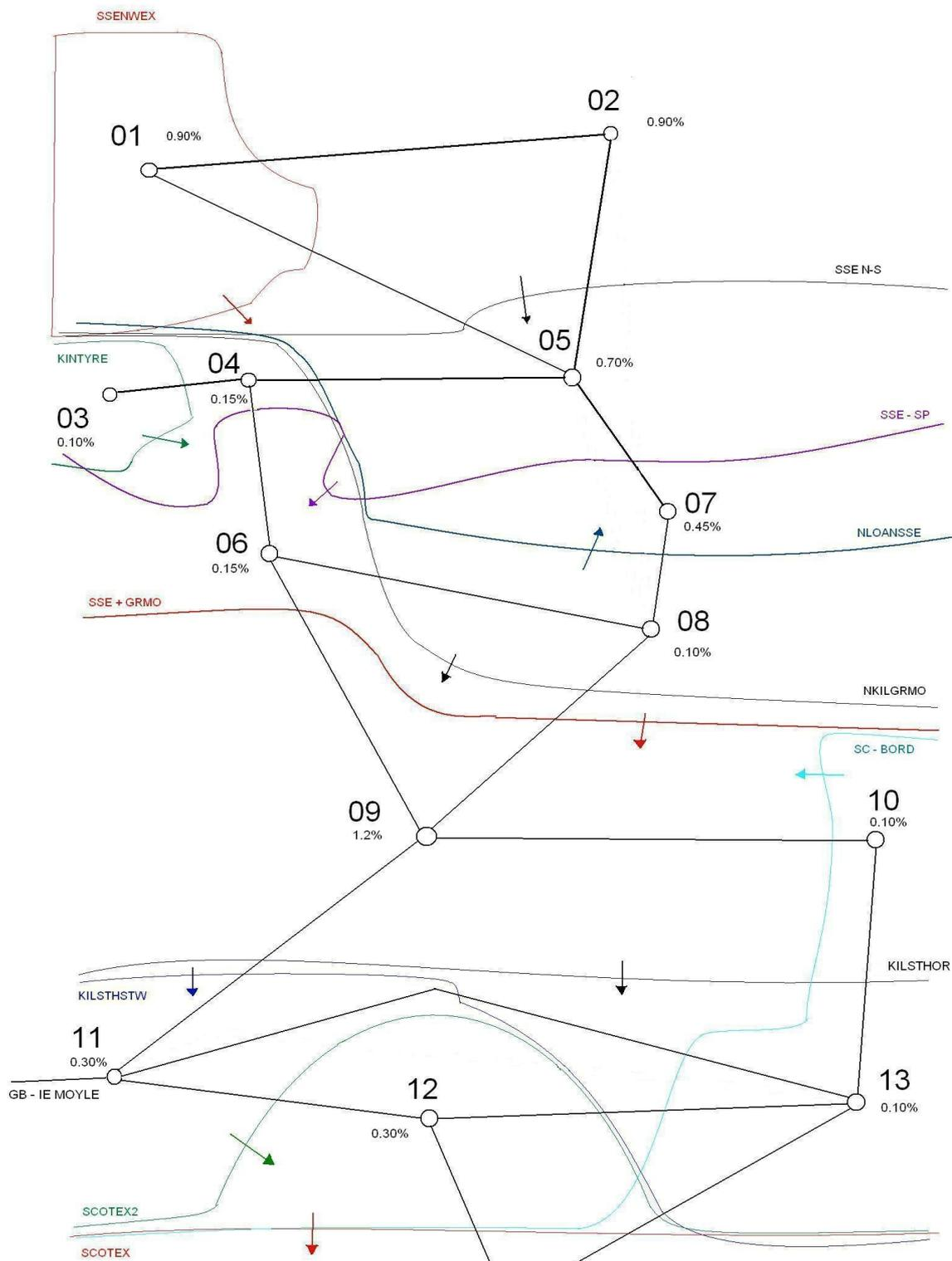
Figure 4: Transmission system (Scotland) model represented by nodes and zones to determine constraint boundaries<sup>11</sup>
