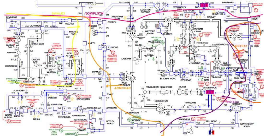
159. During periods of high output from Thames Estuary generation with exports or low imports on the IFA the loss of a double circuit route from the Thames Estuary will result in unacceptable loading of the remaining circuits. Imports from Netherlands on BritNed during such periods (loop flows) would exacerbate the existing issues.
