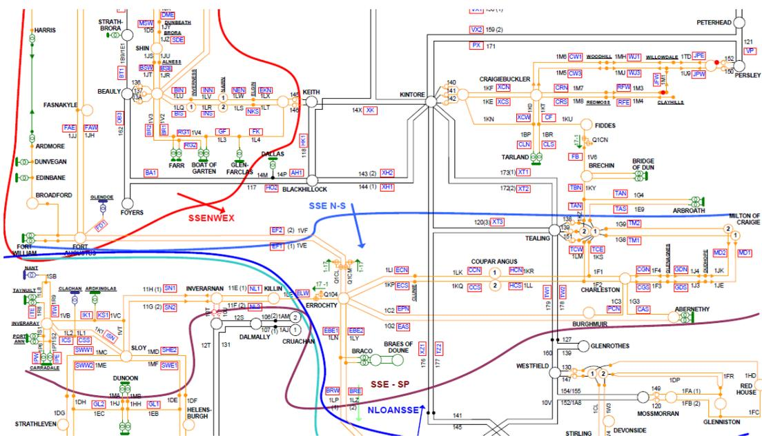
142. The boundary is used to capture all issues associate with high transfers from wind generation combined with generation at Peterhead. The loss of either of the 275kV routes (shown in black) which the boundary crosses can lead to unacceptable overloads on the remaining circuits.
