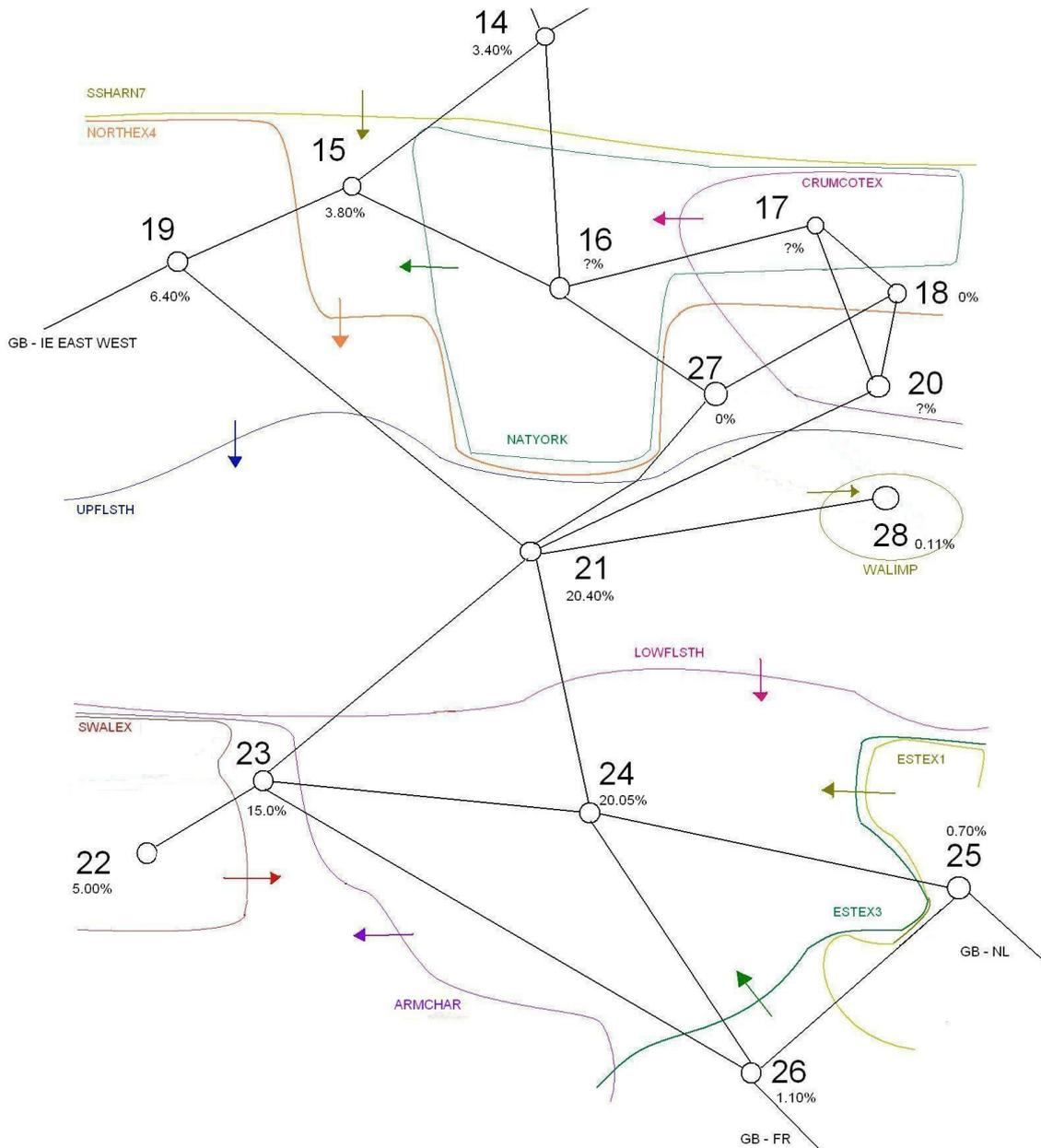
**Figure 5: Transmission system (England and Wales) model represented by nodes and zones to determine constraint boundaries**
