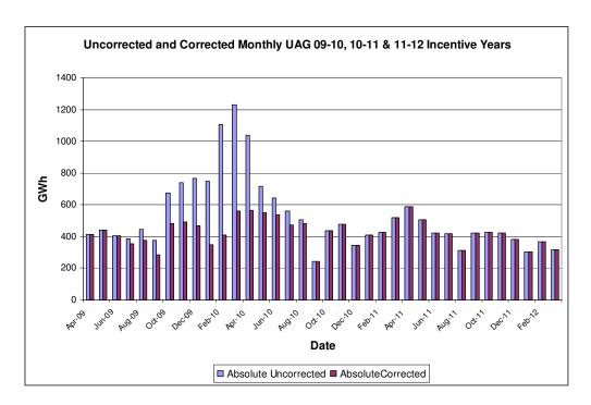
273 It can be seen that the level of corrected UAG has stayed broadly within the same range over the three year period. Clearly the uncorrected level varied significantly; this was due to two meter errors, as described below.
