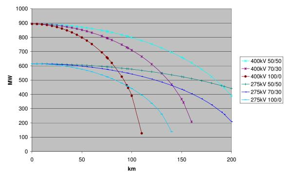
Maximum real power transfer in 275 kV and 400 kV cables with 100/0, 50/50 and 70/30 reactive compensation split between onshore and offshore
