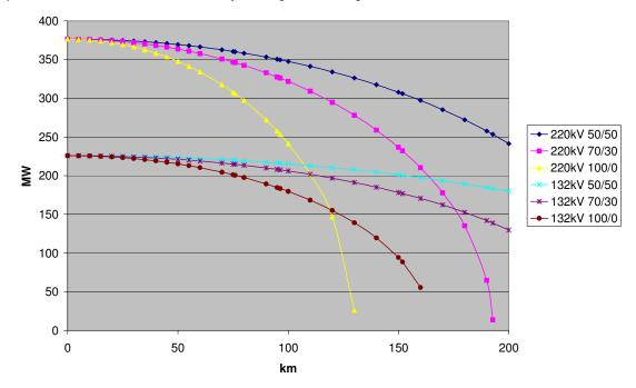
Maximum real power transfer in 132 kV and 220 kV cables with 100/0, 50/50 and 70/30 reactive compensation split between onshore and offshore.
