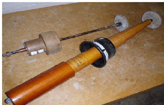
Figure 5.4B – Test Bushings for Metal Clad Switchgear
