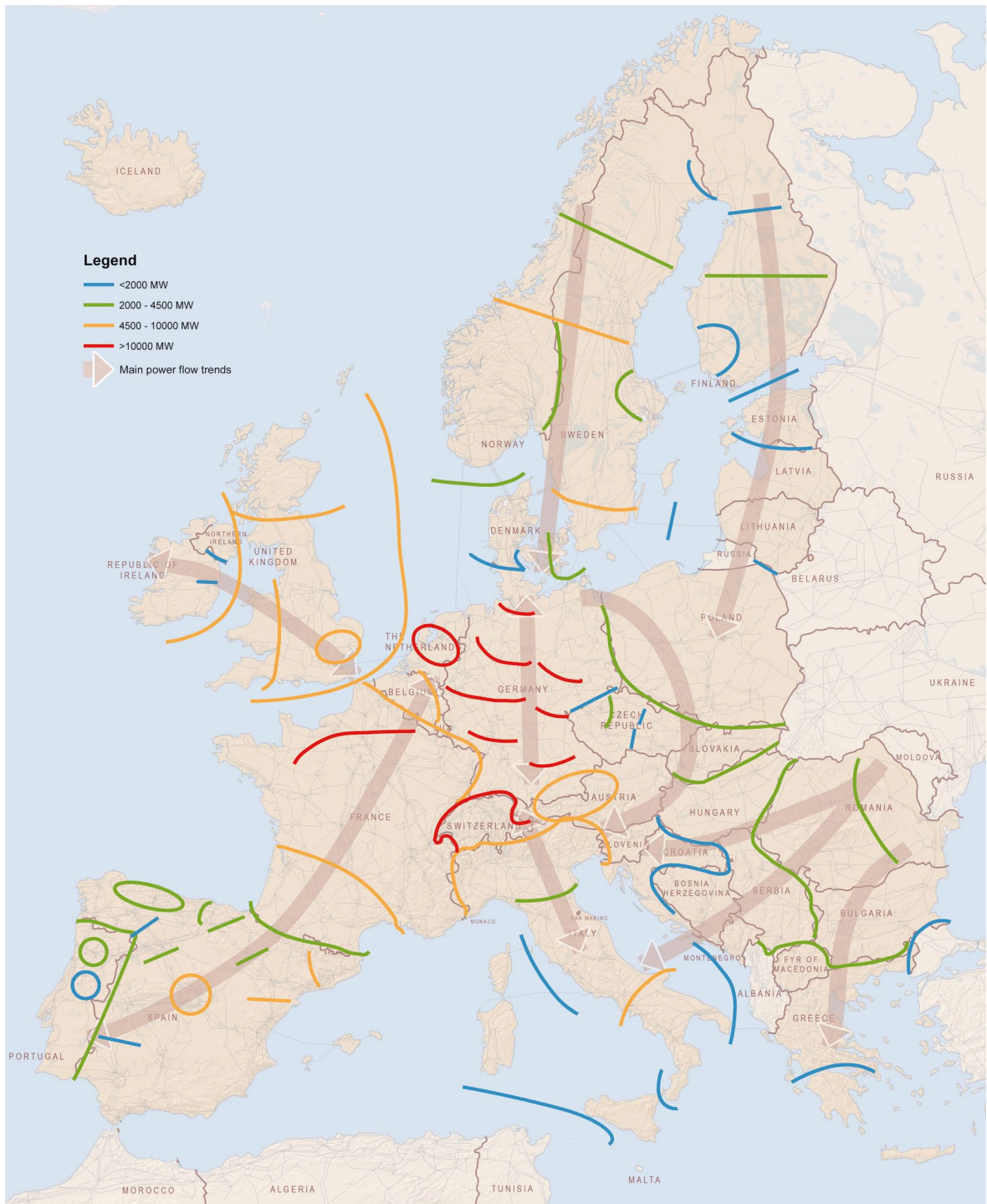
Figure 6.5: Bulk Power Flows related to market integration
