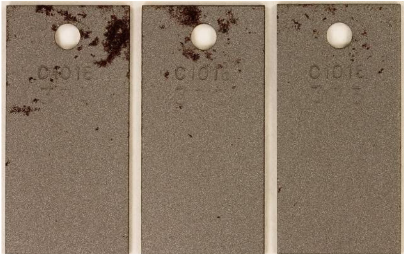
Macrographs of steel corrosion coupons
