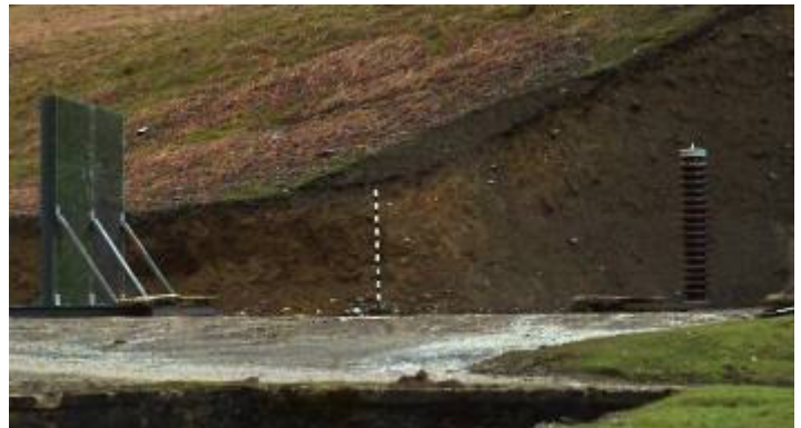
Ballistic testing set up screen distance 10m
