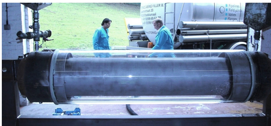
Steel pipe with an acrylic test sleeve to allow for visual during trial installations of the petroleum and polymer replacement filler materials
