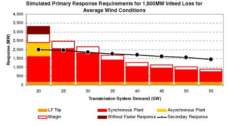
Figure 10: Primary Response Requirements, 1,800MW Loss, Average Wind
