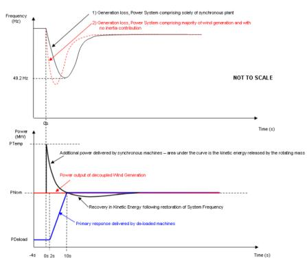
Figure 1: The effect of reduced system inertia on the management of a large infeed loss
