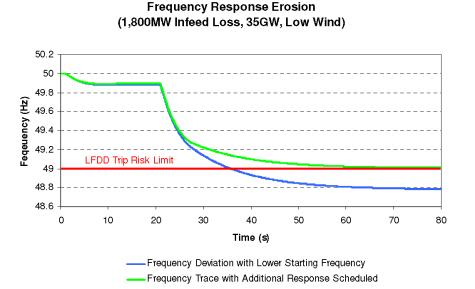
Figure 8: Frequency Response Erosion
