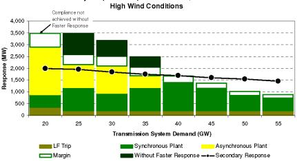
Simulated Primary Response Requirements for 1,800MW Infeed Loss for
