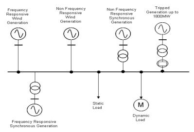
Figure 4: Model used to assess Frequency Response requirements
