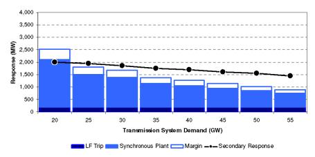
Figure 9: Primary Response Requirements, 1,800MW Loss, Low Wind
