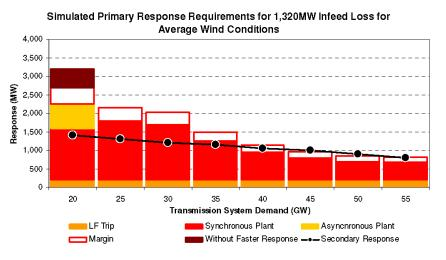
Figure 14: Primary Response Requirements, 1,320MW Loss, Average Wind
