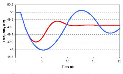
Using Faster Response — Using Primary Response Delivered in 10 seconds
