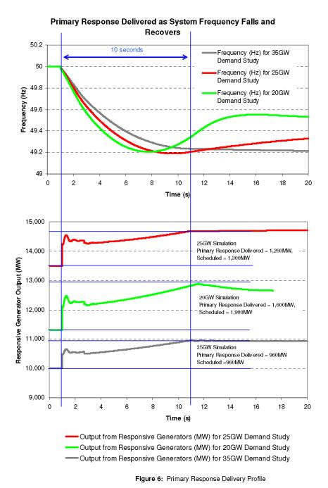
5.5 As the rate of frequency fall increases, the discrepancy between the amount of response scheduled and the response that is delivered at the time required increases. This means that as the rate of frequency fall increases such that it interacts with responsive generators ramping, the requirement for primary Frequency Response increases in line with the assumed ramp rate as well as with the change in system characteristics.
