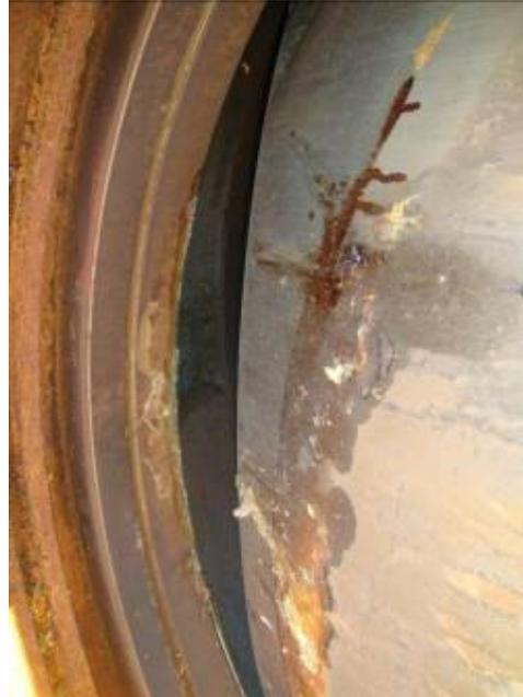
Fig 4 – Distribution of hardened sealant on the inner sealing face
