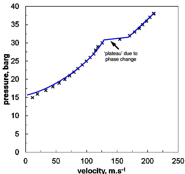
Figure 6 Typical decompression vs velocity plot
