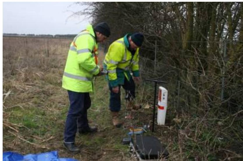
Connecting AC Voltage and Current Readings at the test post at Stallingborough power station
