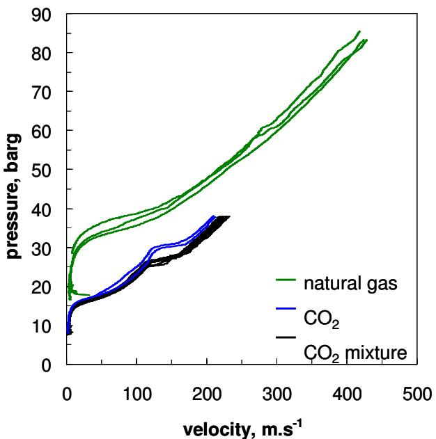
Figure 7 Summary of shock tube test data
