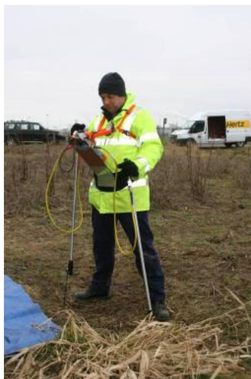
MC Miller Candidate device with prototype AC CIPS module and measurement probes attached during field trial at Stallingborough power station
