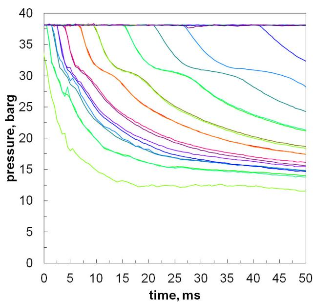
Figure 5 Typical shock tube pressure vs time plot
