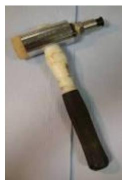
Hammers used for impact testing
