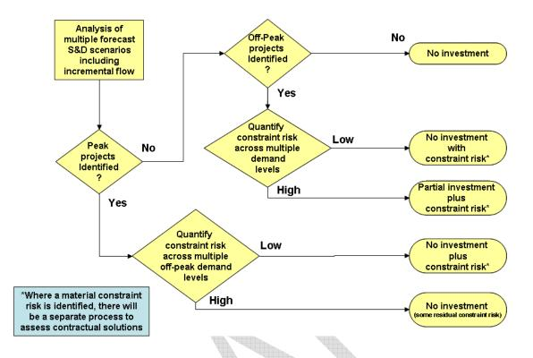
The following diagram outlines the high level process for considering investment versus contractual solutions in relation to exit capacity.
