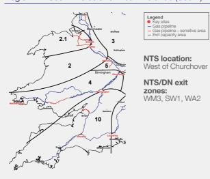
Exit capacity availability is highly sensitive to Milford Haven flows. Low Milford Haven flows result in reduced South Wales pressures, which limit capacity. High Milford Haven flows result in reduced pressures in the West Midlands which may limit capacity.
