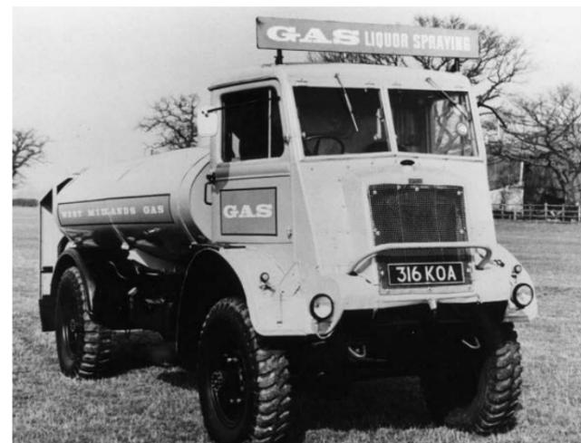
**Figure 53. A tanker used by the West Midlands Gas Board to spray liquor on a farmer's field. Source: National Grid Gas Archive.**
