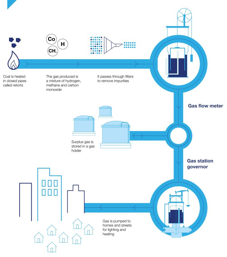
This diagram shows how gas was made from coal. You can see a video of the process in action in the 1960s **here**.
