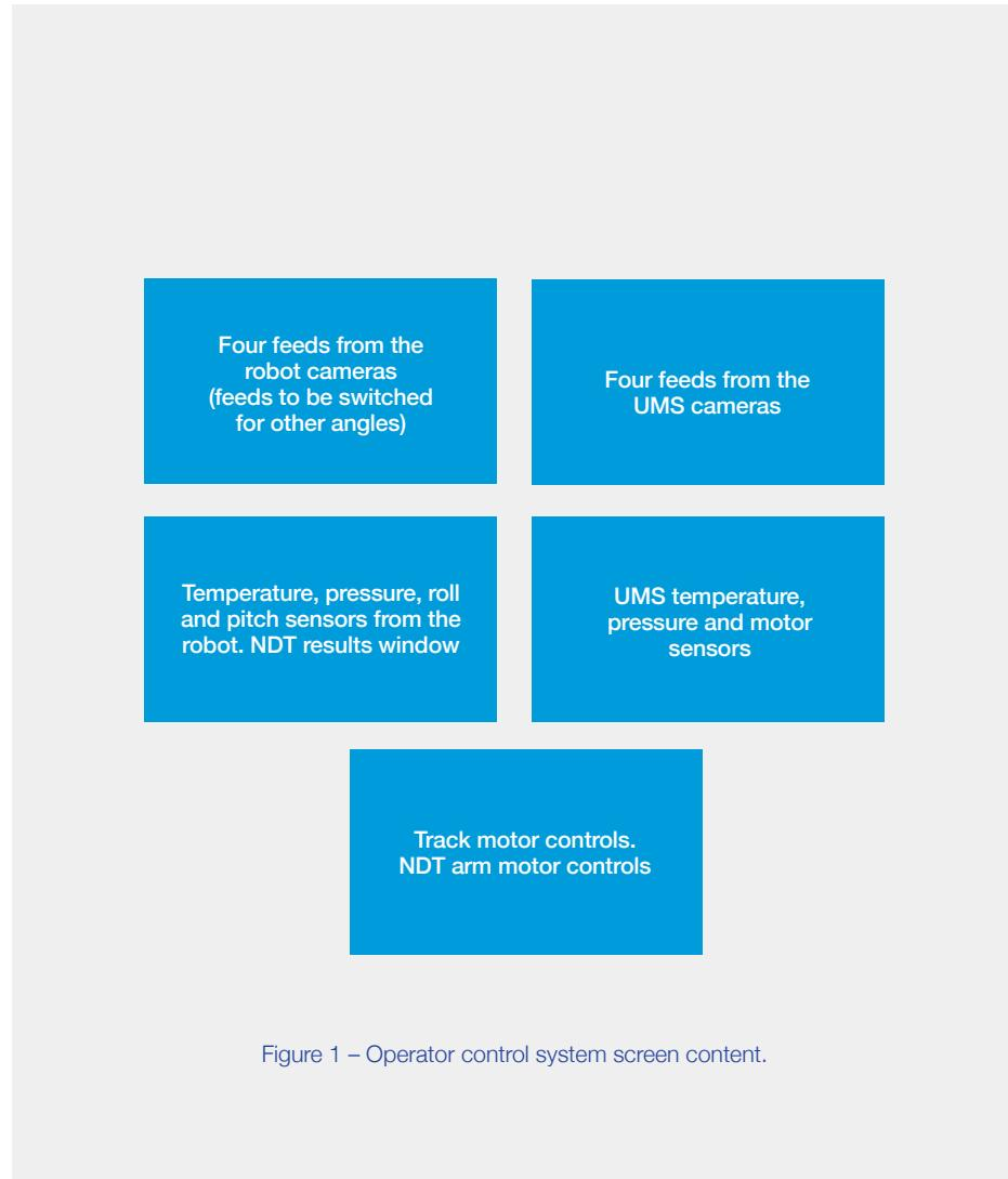
Figure 1 – Operator control system screen content.
