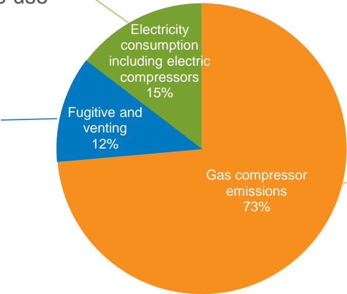
The emissions produced as a result of venting the network to allow access e.g. to perform maintenance; and leaks from assets such as valves
