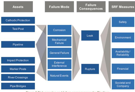
Figure 3 Risk mapping and failure consequences for Pipelines
