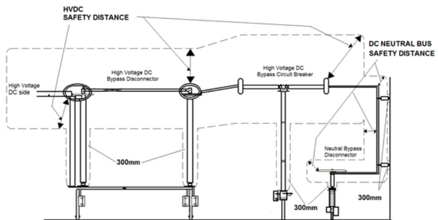
Where the HVDC Bypass Circuit includes only a Bypass Disconnector
