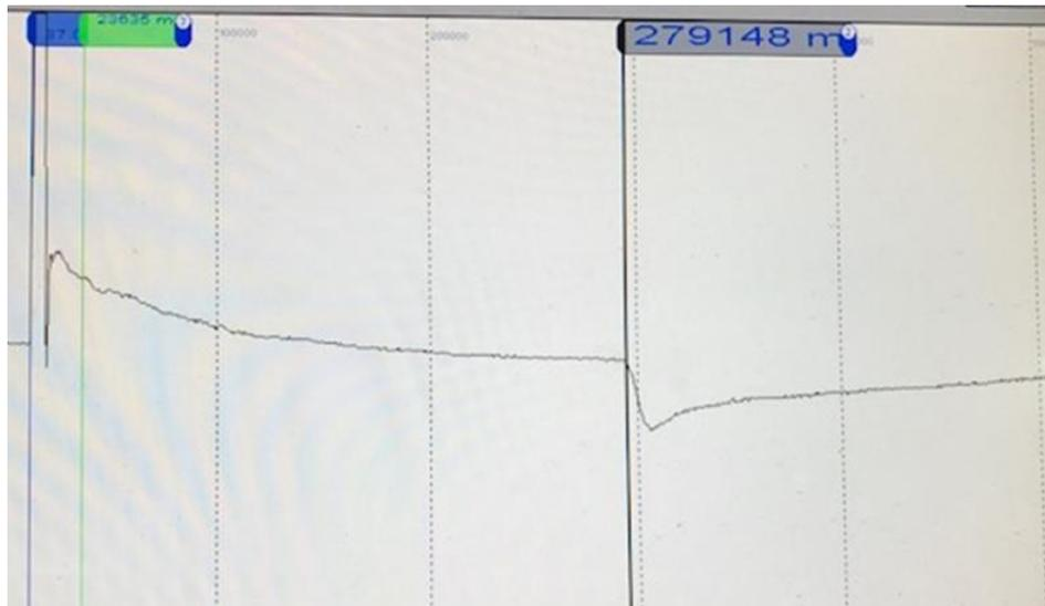
**Figure 1: Example TDR trace from a defective cable**
