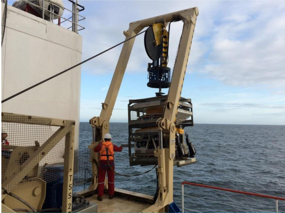
**Figure 2: A Typical ROV being launched**
