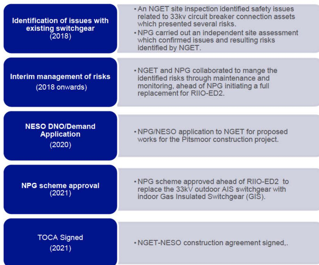
Despite identifying asset health issues related to our switchgear (circuit breakers) in 2018, NGET could not trigger standalone asset replacement works as the metalclad infrastructure is shared with NPG and their switchgear would also need to be replaced as part of a coordinated solution.
