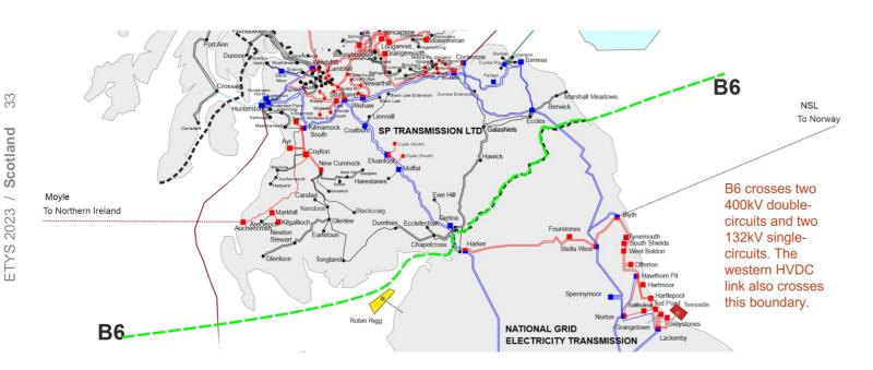
Across all FES, there is an increase in the power transfer requirements from Scotland to England due to the connection of additional generation in Scotland, primarily onshore and offshore wind.
