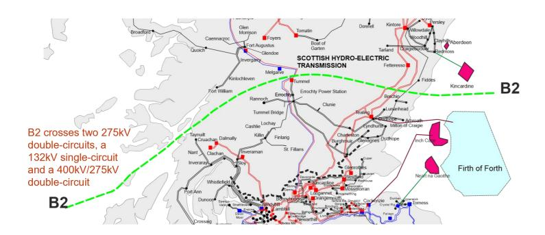
The generation behind boundary B2 includes both onshore and offshore wind, with the potential for additional pumped storage. Thermal generation lies between boundaries B1a and B2, as do several offshore windfarms and proposed future HVDC interconnection to Norway.
