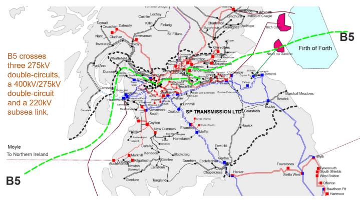
In all the scenarios in the FES, the power transfer through boundary B5 increases because of the significant volumes of generation connecting north of the boundary, including all generation above boundaries B0, B1a, B2 and B4. This is primarily onshore and offshore wind generation.
