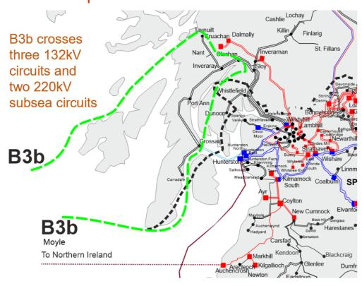
The generation within boundary B3b includes both onshore wind and hydro generation, with the prospect of further wind generation resource and the potential for marine generation being connected in B3b in the future, triggering the requirement for future reinforcement of this network.
