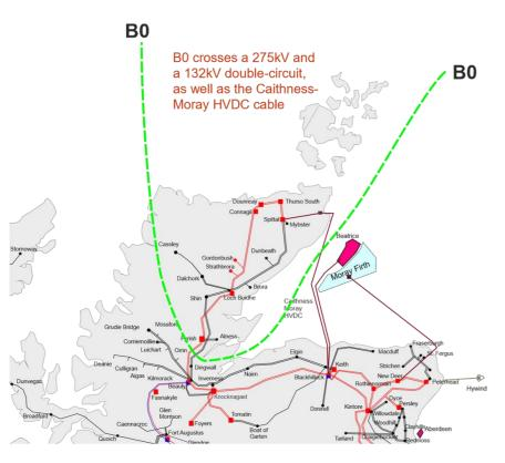
The power transfer through B0 is increasing due to the substantial growth of renewable generation north of the boundary. This generation is primarily centred around both onshore and offshore wind. There is also the prospect of new marine generation resource in the Pentland Firth and Orkney waters in the longer term.
