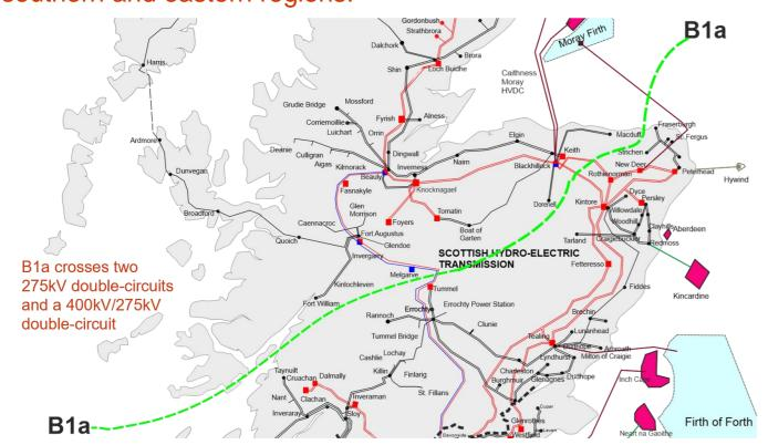
New renewable generation connections north of the boundary are expected to result in a significant increase in export requirements across the boundary, especially along the Beauly – Denny circuit. All generation north of boundary B0 also lies behind boundary B1a.
