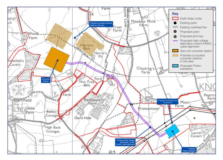
The high voltage alternating current cables would run into the proposed converter station site located to the east of Saxmundham, and to the south of the B1119. Converter stations convert alternating current which transmits power into homes and businesses, into direct current which transports power over longer distances, and vice versa.
