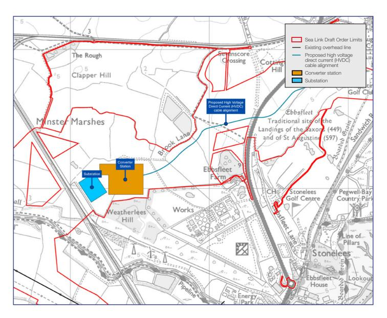
From the transition joint bay, the high voltage direct current (HVDC) cable would pass under the A256/ Richborough Way and continue west for around 2 km towards the proposed substation.
