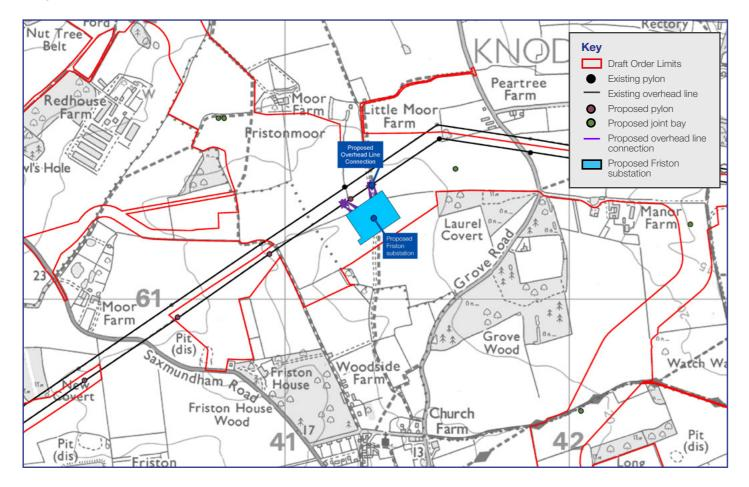
The proposed Friston substation would be located immediately to the north of the village of Friston. It would be constructed using gas insulated switchgear technology with a footprint of up to 16,800 square metres.
