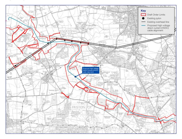
The high voltage direct current underground cable would leave the converter station site and run in an easterly direction for approximately 10 km, continuing to the transition joint bay which is the underground infrastructure needed to transition onshore cables to offshore.
