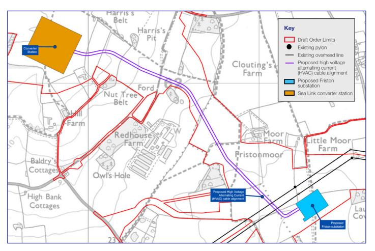
From the substation, there would be a stretch of high voltage alternating current (HVAC) underground cable running northwest, south of the B1119 and north of the B1121, towards the converter station (see above). The HVAC cable stretch would be approximately 1.7 km in length.
