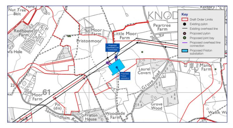
The proposed Friston substation would be located immediately to the north of the village of Friston, adjacent to and to the south of the two existing 400 kilovolt (kV) overhead lines, which run parallel from Sizewell (approximately 6 km to the east) and Bramford substation (approximately 35 km to the south west).
