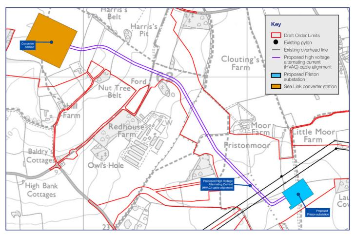
From the proposed substation, there would be a stretch of high voltage alternating current (HVAC) underground cable running northwest, south of the B1119 and north of the B1121, towards proposed converter station. The HVAC cable stretch would be approximately 1.7 km in length.
