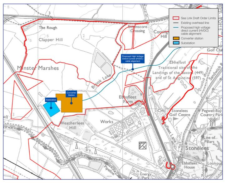
From the transition joint bay, the approximately 2 km HVDC cable would pass under the A256/Richborough Way and continue west towards the proposed substation (outlined on p.50).
