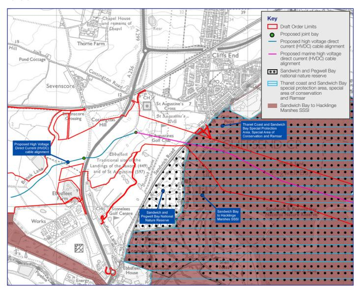
The proposed landfall is located within Pegwell Bay, to the south of the settlement of Cliffsend. The high voltage direct current (HVDC) cables would cross under Sandwich and Pegwell Bay National Nature Reserve, Sandwich Bay to Hacklinge Marshes Site of Special Scientific Interest (SSSI), Thanet Coast and Sandwich Bay Special Protection Area and Ramsar, Sandwich Bay Special Area of Conservation, Sandwich Road, St Augustine's Golf Club and Stonelees Golf Course.
