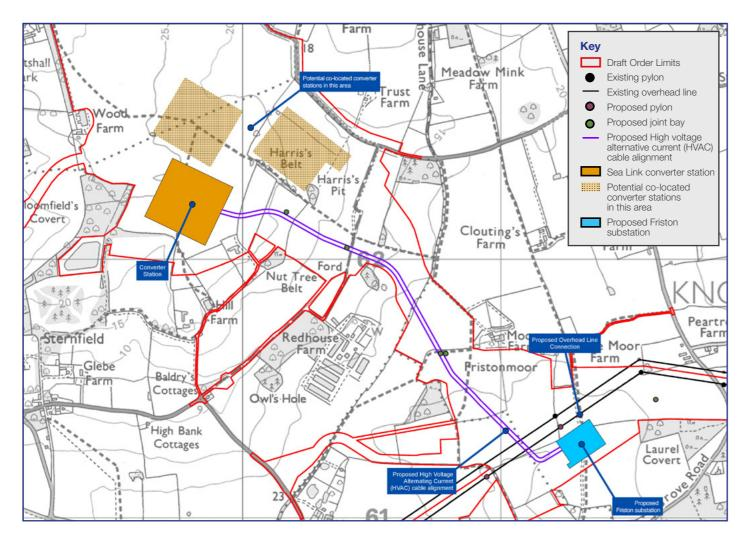
The alternating current cables would run into the proposed converter station site located to the east of Saxmundham, and to the south of the B1119. A single converter station would be required for Sea Link.
