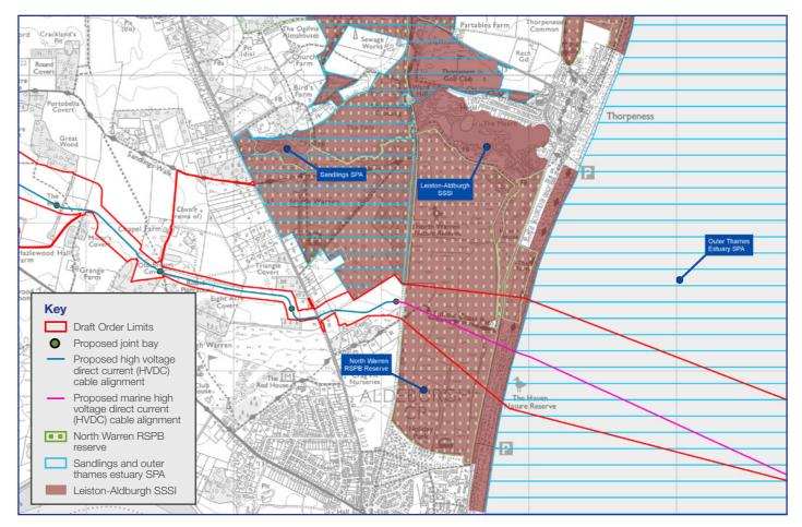
The transition joint bay (TJB) would be located to the north of Warren Hill Land and south of the Sandlings Special Protection Area. The TJB would be approximately 900 metres inshore from the landfall point. At the TJB, the high voltage direct current cable would transition from onshore to offshore technology.
