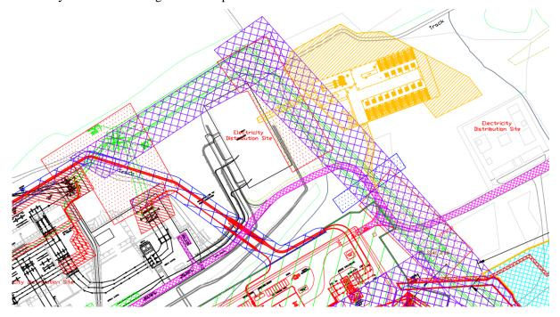
Figure 9: OHL and pylons to be removed and CDM areas required for safe removal of assets. Yellow area is Harmony Energy BESS
