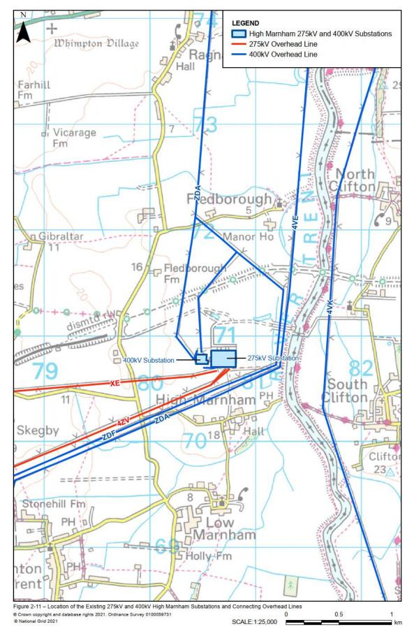
Figure 2-11 – Location of the Existing 275kV and 400kV High Marnham Substations and Connecting Overhead Lines
