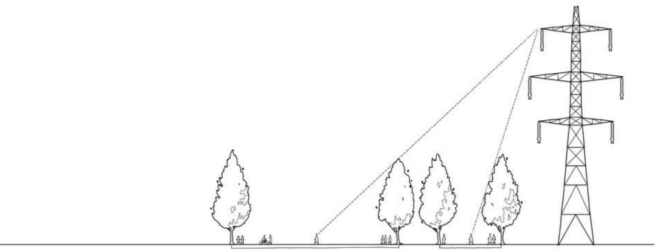
Taller trees are needed to create a similar effect closer to the pylon. However, there are constraints on the size of planting in close proximity to the pylons and lines.
