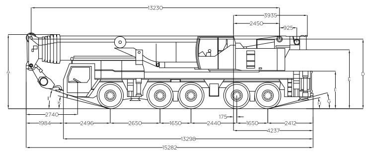
Side elevation - 200 te mobile crane
