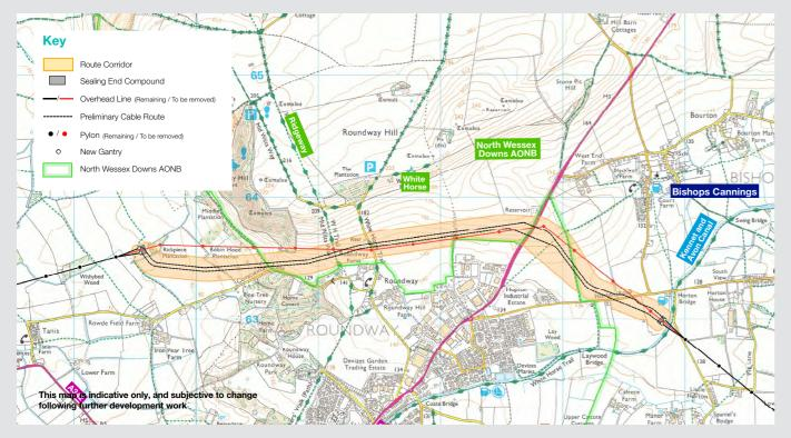
**The North Wessex Downs** project will replace 4.4km of overhead line close to the Millennium White Horse. north of Devizes in Wiltshire, with an underground cable, permanently removing up to 13 pylons from the landscape.
