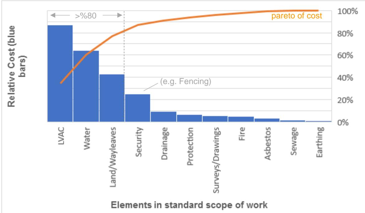
The figure shows that there are 3 main cost drivers within a site separation scheme: LVAC supplies, water services and land purchase / wayleaves. As described in Table 1, these costs are also some of the most variable. Fencing is also a significant cost driver, but is not required at every site.
