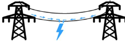
SCL is also used as a description of the strength of the system. When SCL is high we say ‘the system is strong’ and when the SCL is low (as is the case in a system with a high penetration of renewable energy) we say ‘the system is weak’. The strength of the system is a key factor in how stable the system is when it experiences a fault. Table A1 shows how system stability is affected by different levels of SCL.
