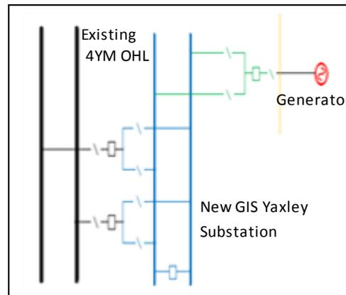
Figure 13: Progress Power Connection and SLD
