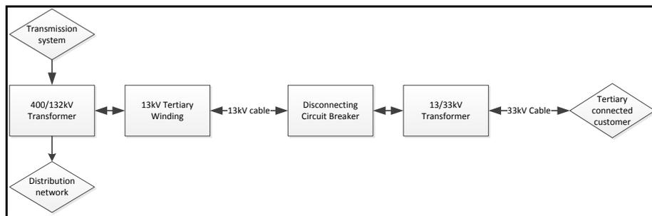
*Figure 8: Typical Arrangement for Tertiary Connected Generation*
